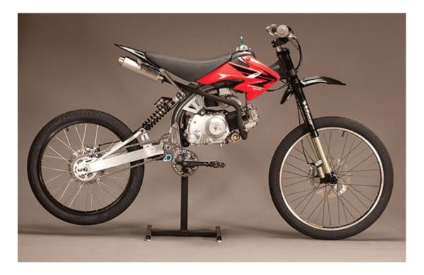
Motoped is a DIY motorized bike kit that you assemble yourself using a XR50/pitbike engine and standard mountain bike components. It uses a Honda xr50 or chinese pitbike engine and downhill mountain bike parts mounted to a custom frame and swing arm.
